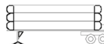
COMPRESSED HYDROGEN TUBE TRAILER
