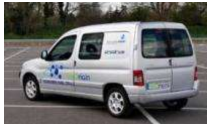
10kW FC Hybrid delivery vehicle with 300km range, -20/+40°C 3min refuel, no loss of capacity
