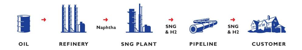
The Gas Company manufactures synthetic natural gas (SNG) from naphtha, a byproduct of the oil refining process
