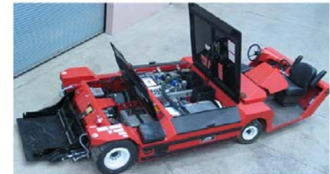
Towbarless Tug with metal hydride storage
