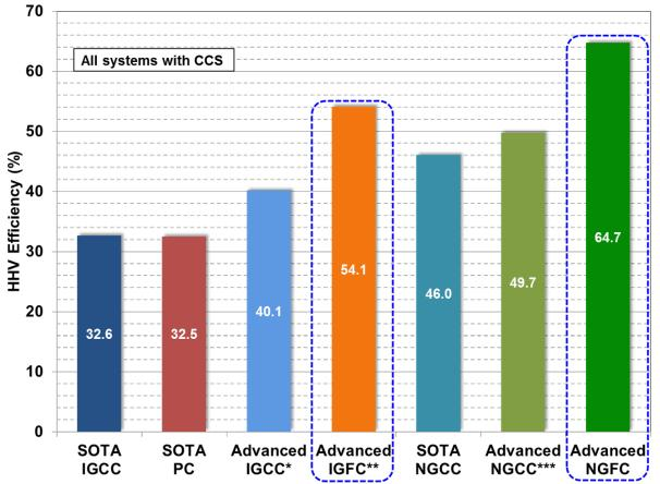
\* Advanced IGCC system includes: coal feed pump, warm gas cleanup, H<sub>2</sub> membrane, advanced H<sub>2</sub> turbine, and ITM
