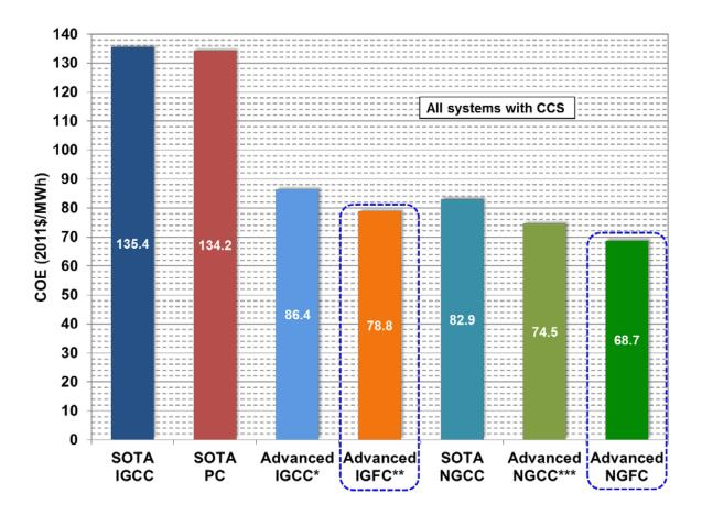
\* Advanced IGCC system includes: coal feed pump, warm gas cleanup,  $H_2$  membrane, advanced  $H_2$  turbine, and ITM
