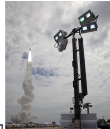
Hydrogen fuel cell powered light tower at Space Shuttle launch
