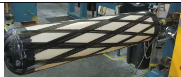
700 bar tank w/ AFP reinforced dome caps
