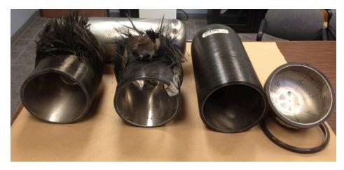
Vessel prototypes have had continuously improving cycle lives. To be soon cryogenically cycle tested
