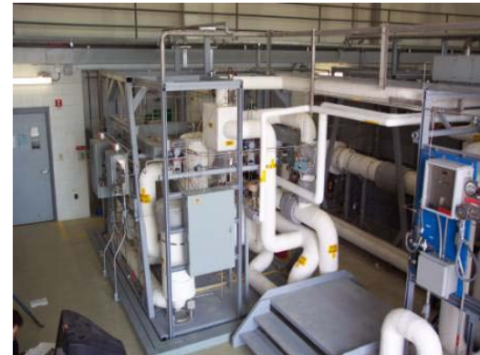
500 kW Diesel Fuel Processor for a PEM Fuel Cell
