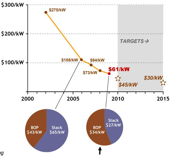
As stack costs are reduced, balance-of-plant components are responsible for a larger % of costs (BOP costs shown here include system assembly & testing).
