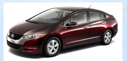
Cruising Range : 620km (390miles) Fuel Cell Stack : 100kW Top Speed : 160km/h (100mph) Pressure of Hydrogen Tank : 35MPa
