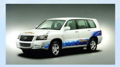
Cruising Range : 830km (520miles) Fuel Cell Stack : 90kW Top Speed : 155km/h (97mph) Pressure of Hydrogen Tank : 70MPa
