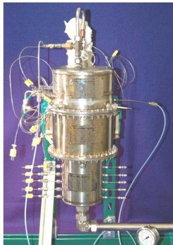
26 kWt JP-8 Fuel Processor for Army PEM fuel cell
