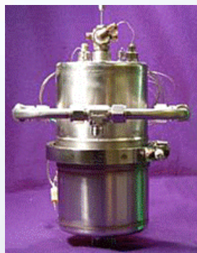
26 kWt JP-8 Fuel Processor for Army PEM fuel cell
