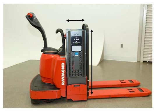
Fuel cell unit in pallet truck
