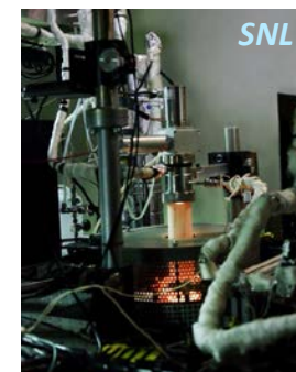
Stagnation flow reactor to evaluate kinetics of redox material at high-T
