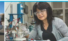
Xiaoping Wang of Argonne National Laboratory prepares a cell for testing the activity of fuel cell catalysts.
