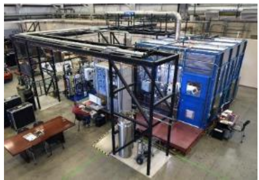
25 kW high-temperature electrolysis @ INL Energy Systems Laboratory
