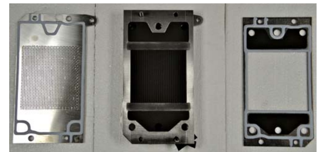
Stack components at INL
