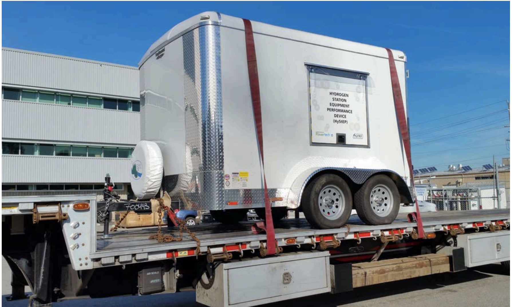
Hydrogen Station Equipment Performance Device(HySTEP) – improve station commissioning
