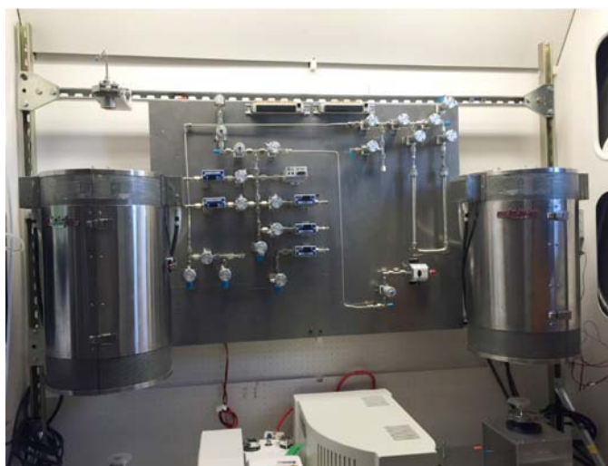
FIGURE 3. Photograph of the existing state of the flowing particle reactor test system
