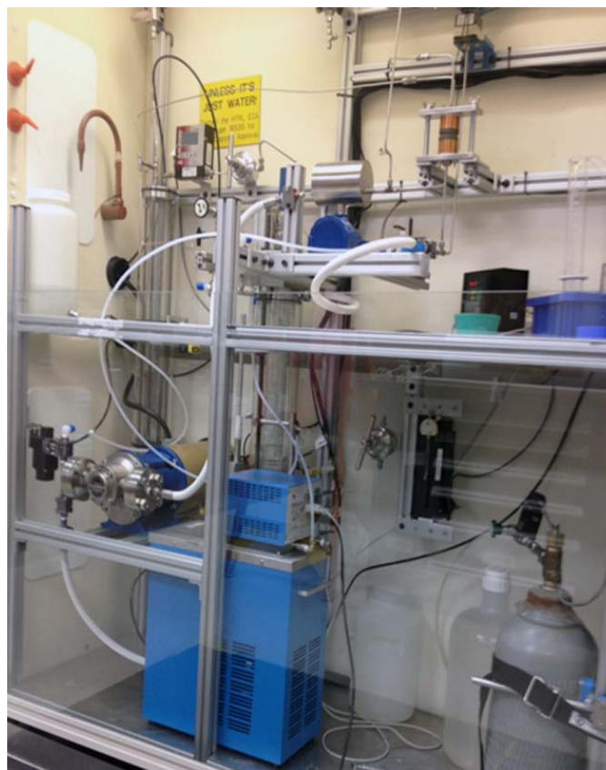
FIGURE 1. Photograph of pressurized button cell test facility
