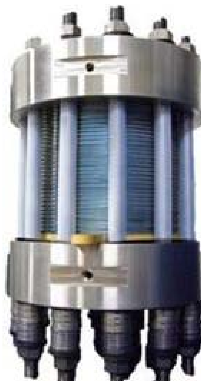
FIGURE 1. EHC 30-cell stack (81 cm 2 design)
