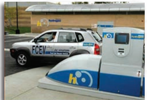
A Hyundai fuel cell vehicle refuels at the Chevron hydrogen fueling station in Chino, CA
