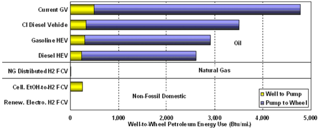
Figure 5. WTW Petroleum Use of Selected Vehicle/Fuel Systems
