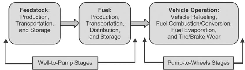
**Figure 1.** Stages Covered in GREET Well-to-Wheels Analysis
