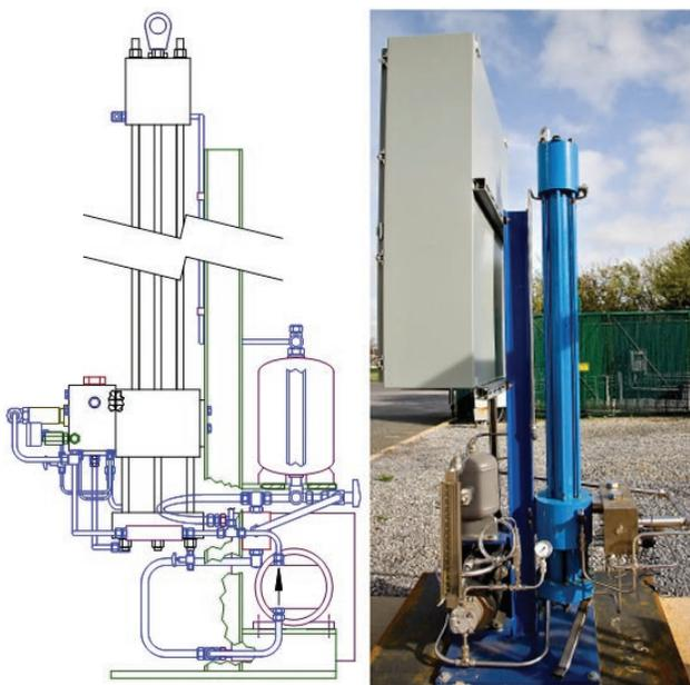
**FIGURE 5.** Novel Compressor Schematic (left); Novel Compressor (right)
