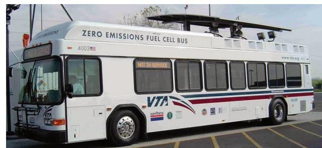
**FIGURE 1.** The Buses at VTA use a Non-Hybrid Fuel Cell System Developed by Ballard Power Systems
