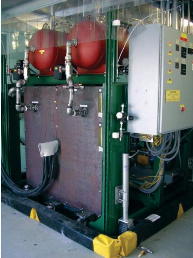
FIGURE 1. Ambient Pressure Plastic Electrolyzer stack
