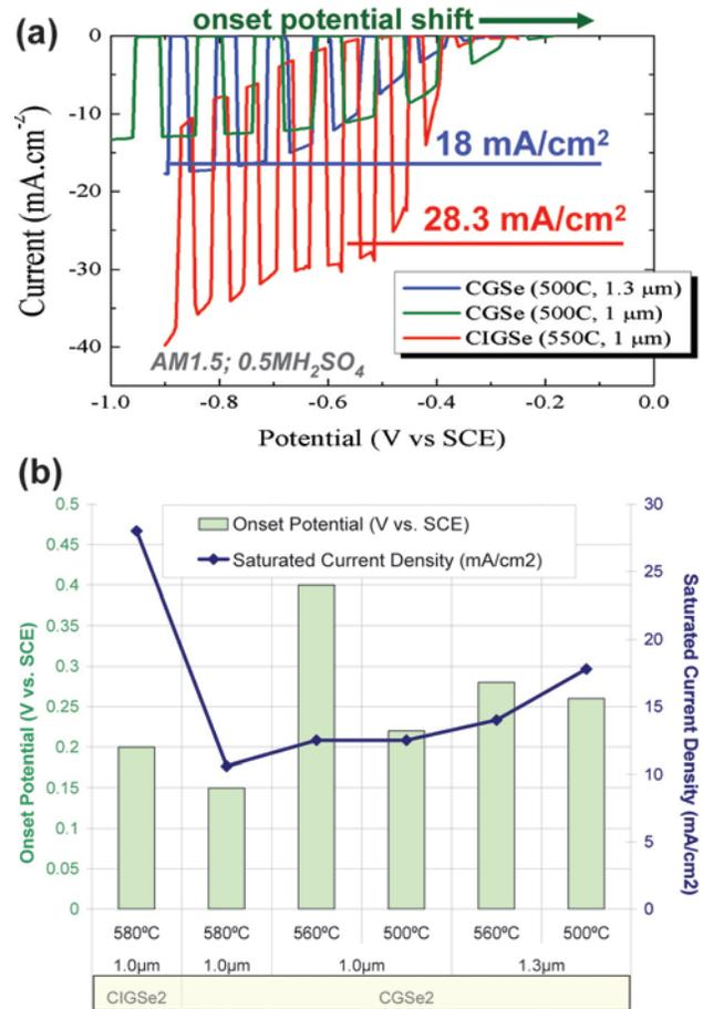
**FIGURE 3.** (a) Light chopped LSV curves showing performance of  $\text{CIGSe}_2$  (red curve) vs. two  $\text{CGSe}_2$  samples (blue and green curves) deposited under different conditions. PEC photocurrent levels and onset potential shifts are noted; (b) Absolute onset potential and saturated photocurrent density values measured on  $\text{CGSe}_2$ -based PEC electrodes fabricated with varying deposition temperature and thickness.
