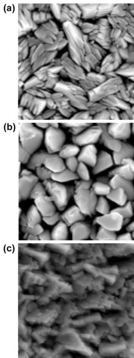
**FIGURE 1.** SEM top views ( $1 \times 1 \mu\text{m}^2$ ) of (a)  $\text{WO}_3$  (2  $\mu\text{m}$  thick), (b)  $\text{Mo:WO}_3$  (2  $\mu\text{m}$  thick), and (c) bi-layer ( $\text{Mo:WO}_3/\text{WO}_3$  - 200 nm/1.8  $\mu\text{m}$ ).
