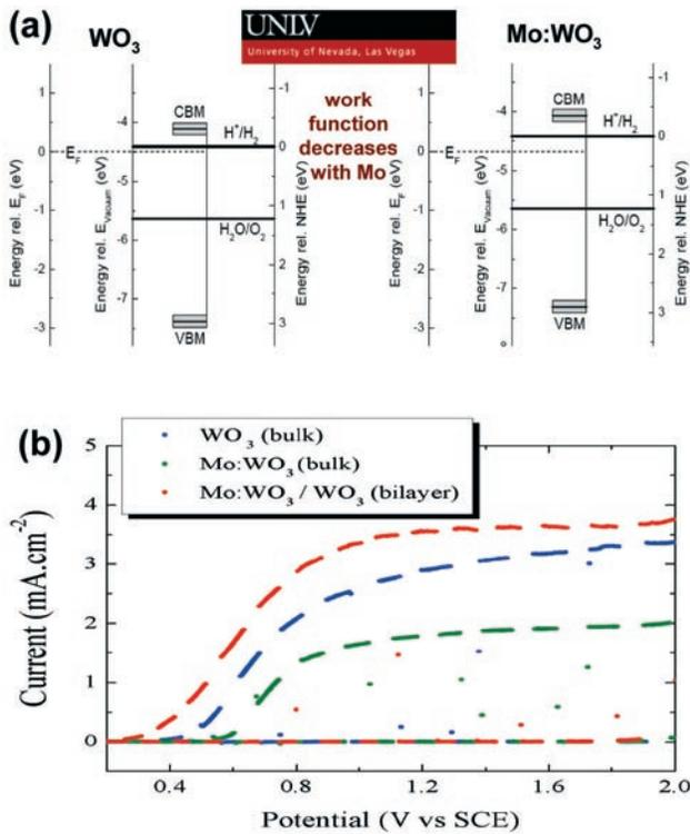
**FIGURE 2.** (a) Band diagrams of  $\text{WO}_3$  and  $\text{Mo:WO}_3$ , obtained from ultraviolet photoelectron spectroscopy and inverse photoemission spectroscopy analyses showing work-function and band-edge shift; (b) Linear sweep voltammetry characteristics of  $\text{Mo:WO}_3$ ,  $\text{WO}_3$ , and bi-layer showing enhanced PEC photocurrents in the bi-layer.
