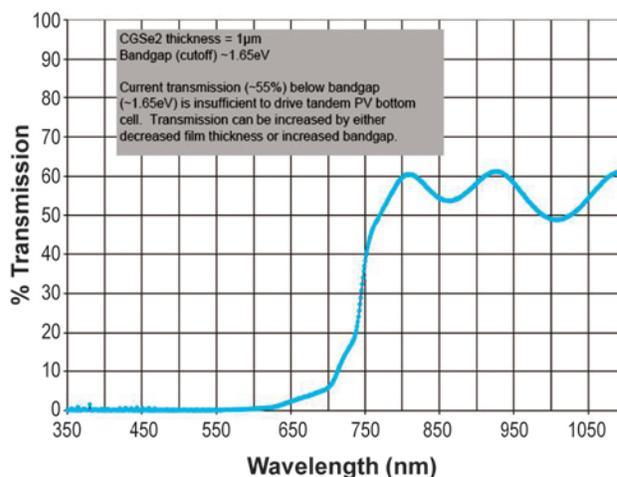
**FIGURE 1.** UV-visible spectra of transmission through a 1  $\mu\text{m}$   $\text{CGSe}_2$  film. Transmission is insufficient to drive a tandem PV bottom cell, necessitating a thinner top film.
