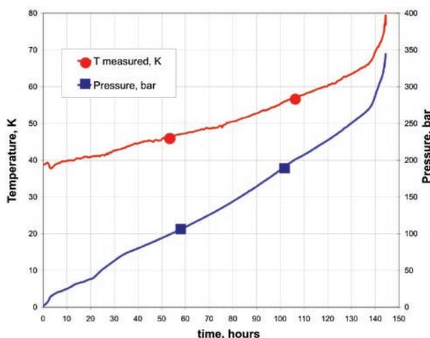
**FIGURE 2.** Pressure and temperature measured inside the vessel during the dormancy experiment.
