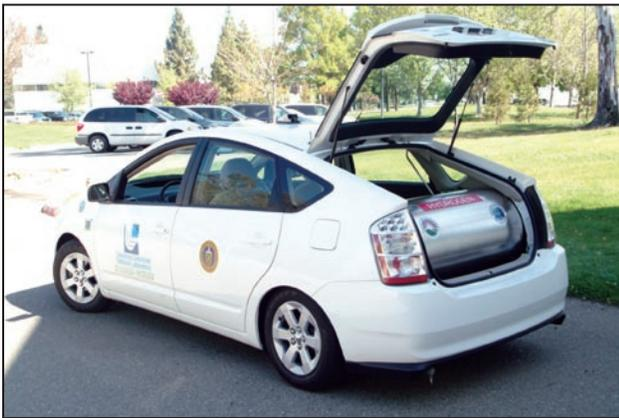
**FIGURE 1.** LLNL experimental hydrogen Prius with the cryogenic-compatible pressure vessel installed in the trunk.
