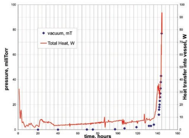
**FIGURE 3.** Pressure in the vacuum insulation (measured) and heat transfer into the vessel (calculated from the measured temperature and pressure, Figure 2) during the 6-day dormancy test.
