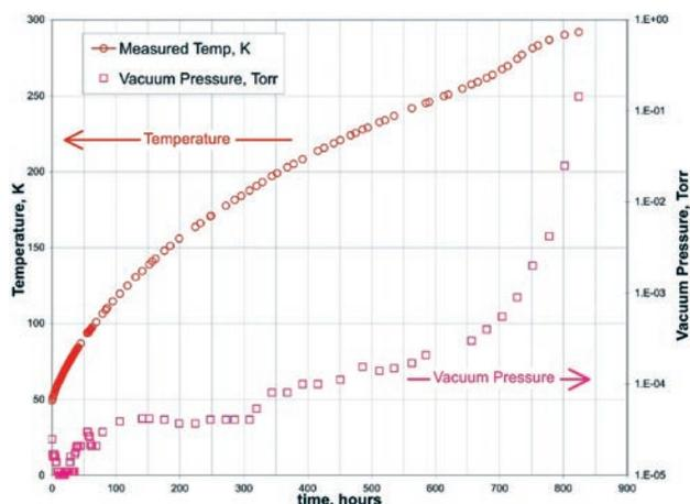
**FIGURE 4.** Vessel temperature and pressure in the vacuum space during a 5-week vacuum stability test.
