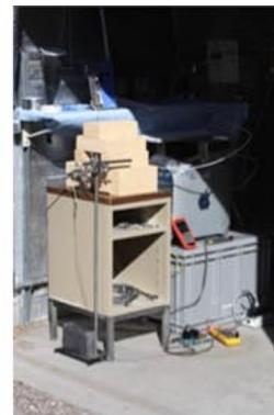
**FIGURE 3.** An open outdoor facility at LANL was used to test packaged, working LANL/LLNL  $H_2$  sensors in flammable mixtures of hydrogen and air.
