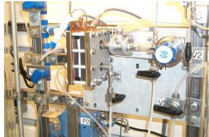
Research-type Electrolyzer (40 cm 2 )
