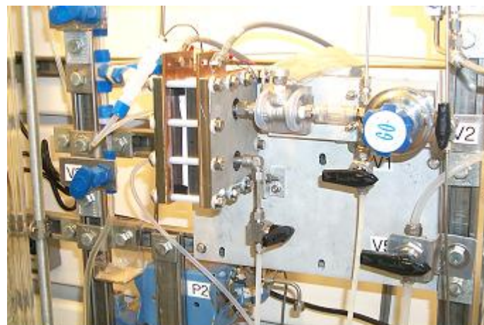
SO 2 -depolarized electrolyzer
