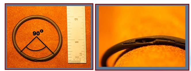
O-Ring Damage 3000 psig Fatigue Test
