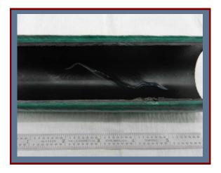
Inside View Showing Rupture of Liner
