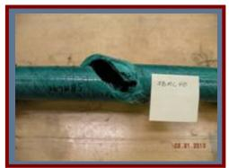
Baseline Flaw 1"x 0.125" 40% Depth No Evidence of Bulging Under Sustained Pressure
