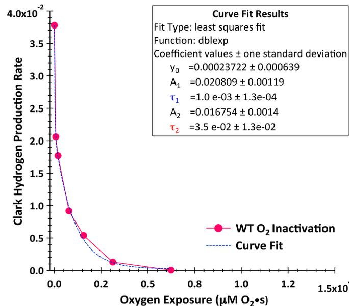
Clark H<sub>2</sub>-Production Rate versus  $\mu\text{M O}_2 \cdot \text{s}$  were plotted, and the results fitted to a bi-exponential-decay curve, according to the equation below. The two inactivation rate constants,  $\tau_1$  and  $\tau_2$ , were estimated for WT and Ca1 cells.
