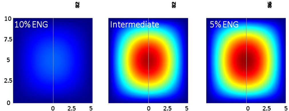
Net volumetric storage of hydrogen vs. time for the three values of thermal conductivity. ( $k = 0.55, 0.32, \text{ and } 0.16 \text{ W/m-K}$  for 10%, Mid-value, and 5% ENG, resp., at 110 K)
