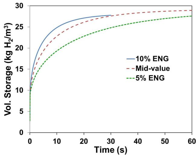
← A pellet compacted to 0.51 g/cm<sup>3</sup> at 140 K and 4 bar (empty) is enveloped in H<sub>2</sub> gas at 80K and 30 bar (refueling)
