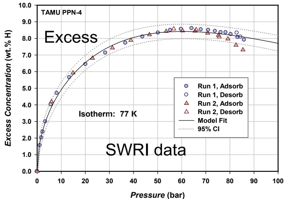
PPN-4(Si) has ultrahigh surface area ( $S_{\text{BET}} = 6470 \text{ m}^2/\text{g}$ ) and is **very stable**. This surface area is one of the highest reported to date for any porous material. Yet, volumetric uptake (**28 g/L**) is low due to extremely low framework density (**0.284 g/cm<sup>3</sup>**) and lack of strong H<sub>2</sub>-binding sites.
