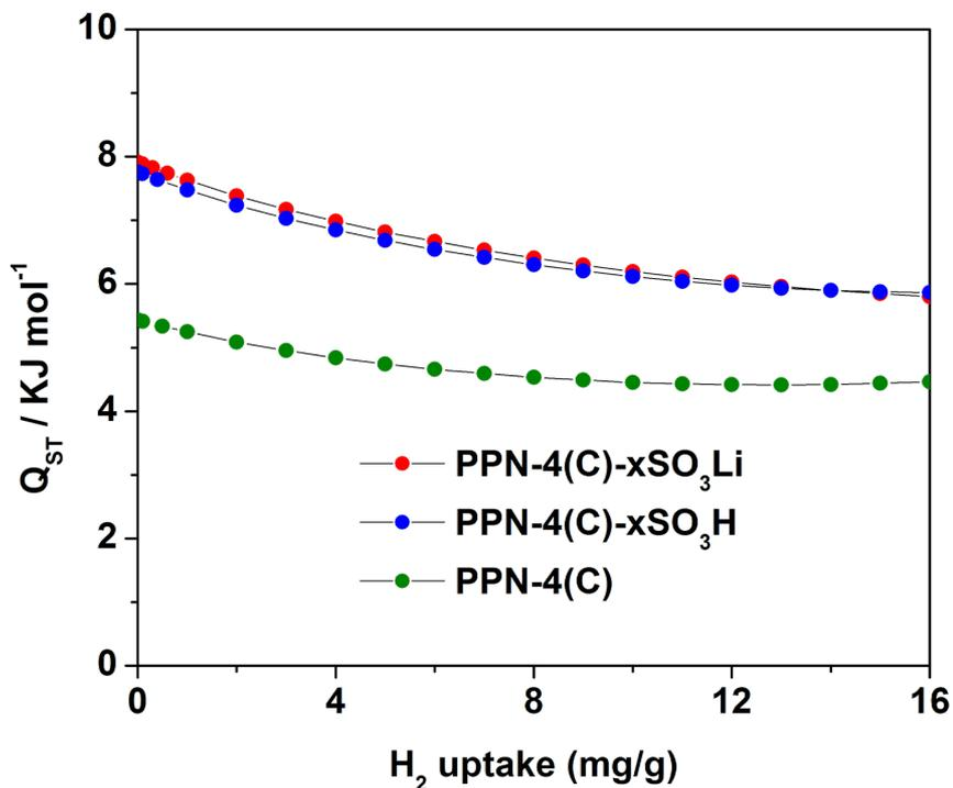
Isosteric heats of adsorption obtained from isotherms at 77 and 87 K. H<sub>2</sub> heat of adsorption has improved by 47% upon post-synthetic modification.
