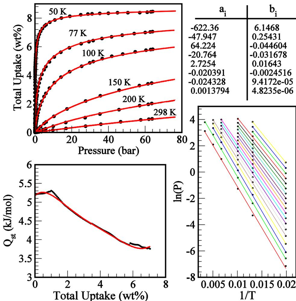
On the left, we show the isotherm data and the corresponding virial-fits.  $Q_{st}$  is around 5.2 kJ/mol initially and then start to decrease down to 4 kJ/mol. These numbers are typical for copper-paddle wheel MOFs. **The initial flat  $Q_{st}$  is a sign that the main adsorption sites are copper sites!**
