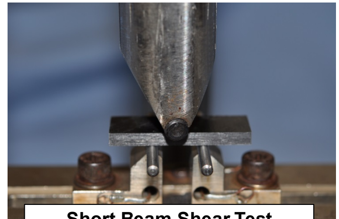
Short Beam Shear Test
