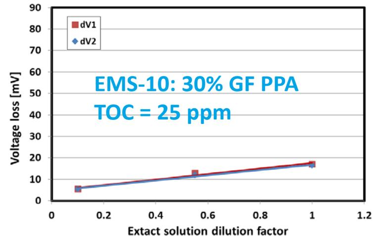
Test conditions: 80°C, 32/32 % inlet RH, 0.2 A/cm<sup>2</sup>,
