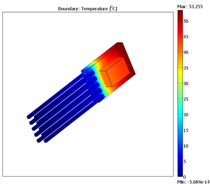
thick wires, no thermal insulation
