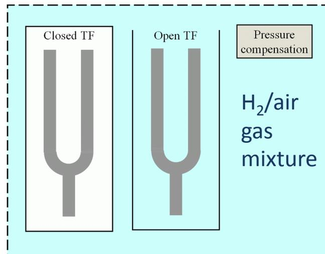
Microresonance technology based sensor
