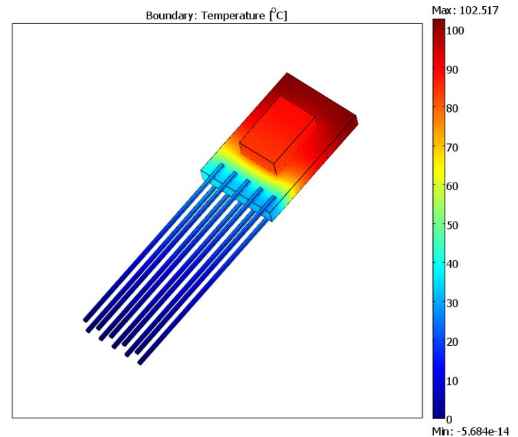
thin wires, with thermal insulation
