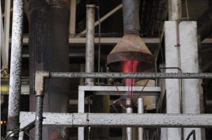
Industrial operations flare or vent hydrogen rich furnace exhaust gas into the atmosphere today
