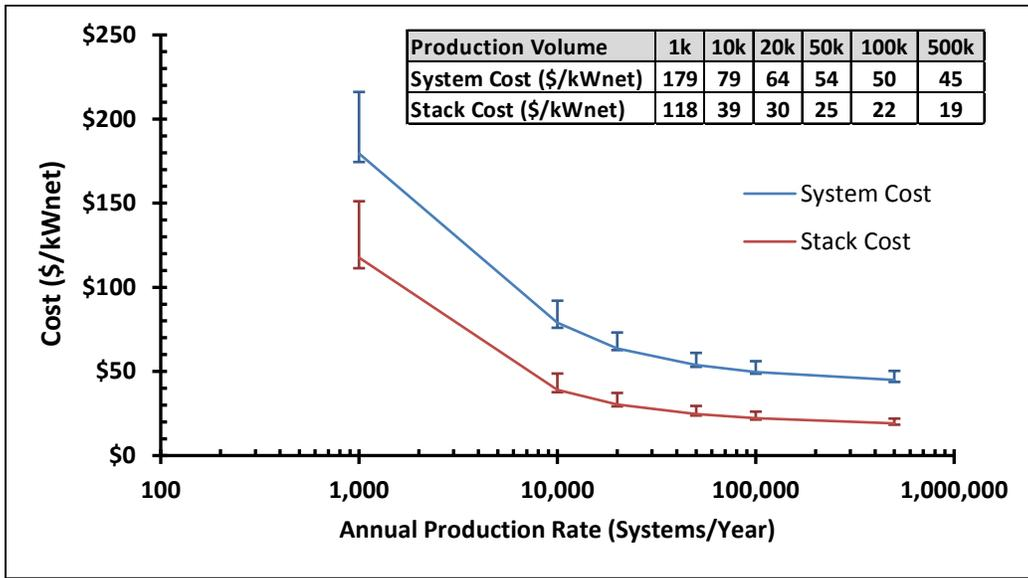
Figure 2. Projected cost of 2017 80-kW<sub>net</sub> transportation fuel cell stacks and systems at 1,000, 10,000, 20,000, 50,000, 100,000, and 500,000 units/year.
