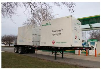
Figure 3: Hydrogen Delivery System Source: Air Products and Chemicals, Inc.
