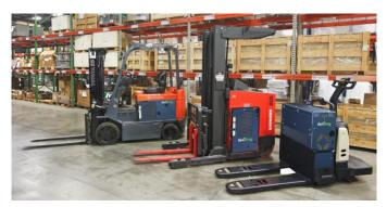
Figure 4: Fuel Cell Powered Forklifts by Plug Power Inc. Source: Plug Power Inc.
