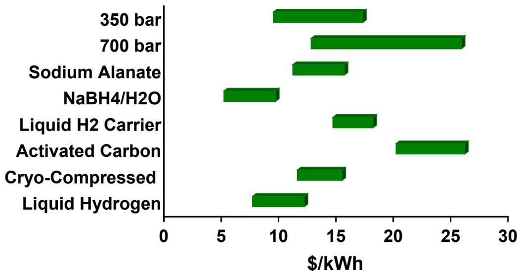
**Figure 3. Estimated range of projected costs during high-scale production (i.e., 500,000 units/year) for several on-board storage systems with usable hydrogen capacities of 5.6 kg. These ranges include the most recent updated results for each system as reported through June 2010.**
