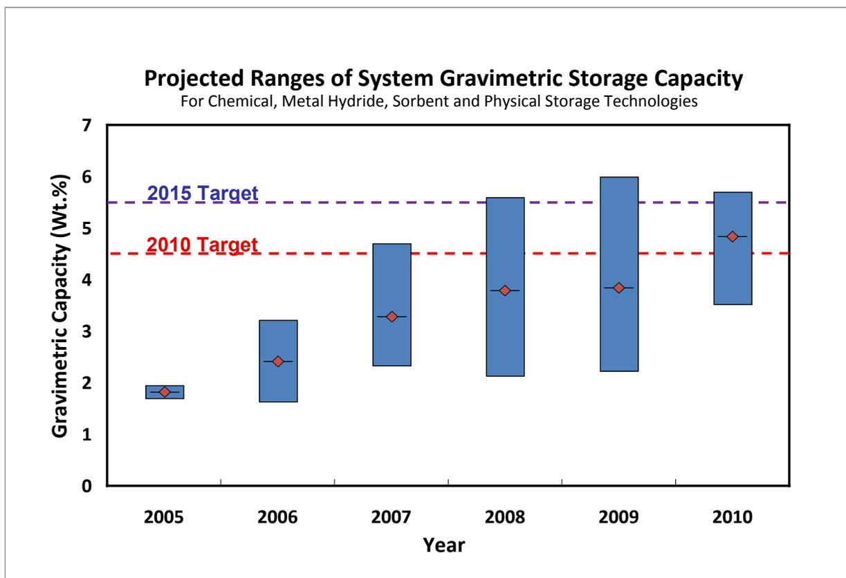
**Figure 1.** Estimates of gravimetric capacities projected for on-board storage systems that can supply 5.6 kg of usable hydrogen as compared to DOE targets (based upon engineering analyses). Note that the plotted data points are the average value for all systems analyzed during each year while the bars correspond to the range of maximum and minimum values obtained in each year. Also note that systems with predicted capacities exceeding the gravimetric targets do not meet other targets.
