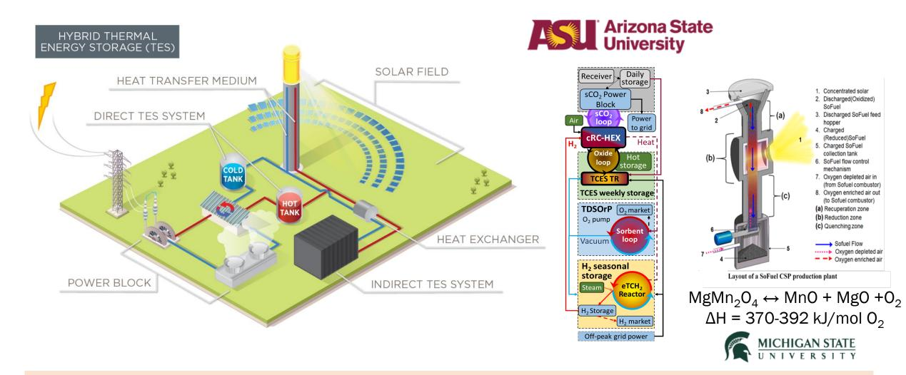
Existing power block at a CSP plant can be leveraged for high value 'indirect' TES via long-duration thermochemical or (renewable) fuels
