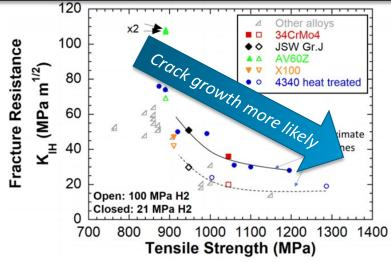
Systematic in situ testing of 9 microstructural variants of a PV steel confirm strong correlation between strength and reduced fracture resistance.
