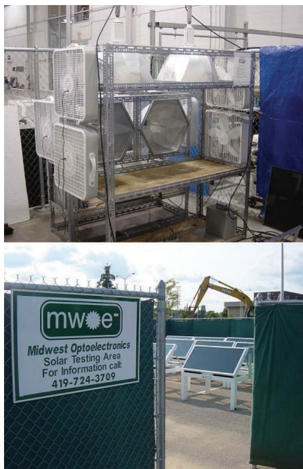
FIGURE 2. (top) Large-area light source for evaluation of 2 ft x 4 ft PEC panel (bottom) Outdoor testing facility for evaluation of arrays of PEC panels outdoor.
