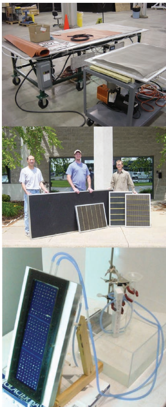
FIGURE 4. (top) Mid-size (2 ft x 3 ft) and large-area (3 ft x 8 ft) laminators used for the encapsulation of substrate-type PEC panels (middle) Solar modules (dummy modules without semiconductor coatings) encapsulated using the laminators (bottom) Small area (4 in x 12 in) substrate-type PEC panel with 5.9 cc/min hydrogen generation rate under 0.92 sun intensity.
