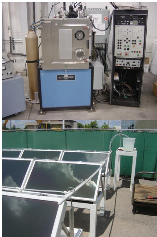
FIGURE 3. (top) Large-area, four-gun sputter deposition systems capable of depositing photocatalyst on 1 ft x 4 ft flexible substrates (bottom) Gas collection system on the superstrate-type PEC panels.
