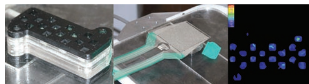
FIGURE 3. Pressure/Flow Measurement Experiment with Example Ceramic Heat Exchanger Plate
