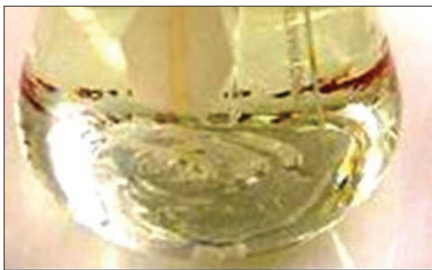
FIGURE 6. Zinc Powder Precipitate using the GTI Electrochemical Cell
