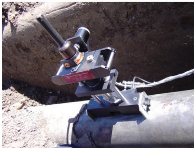
FIGURE 5. ATC SSM Hydrogen Chamber (top) allows conducting five ABI tests on each of six pipeline steel samples (1-inch diameter, 0.375-inch thick) at high hydrogen pressure and at various increasing exposure times using ATC’s portable/in-situ SSM system (bottom)
