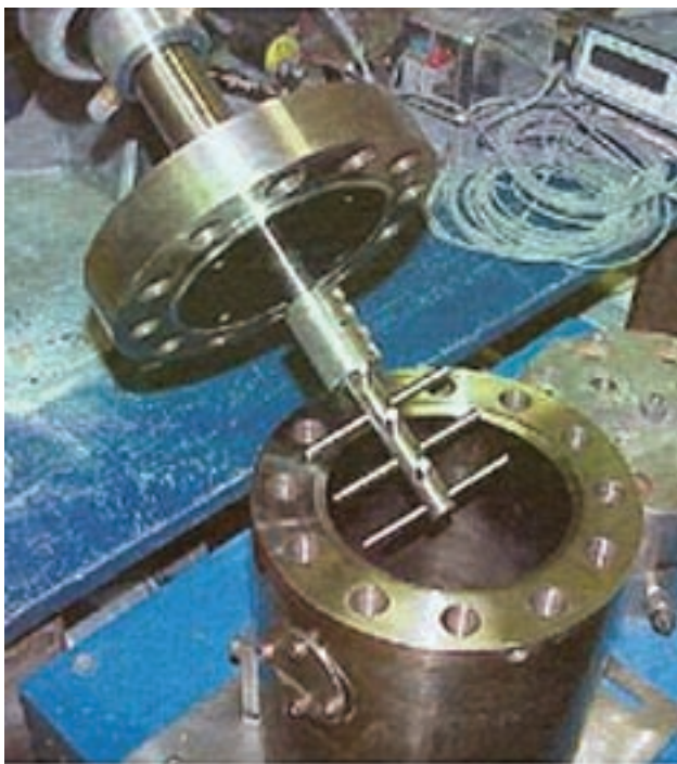
FIGURE 3. Attrition Mill Used to Synthesize 0.5 kg Batches of Complex Hydrides
