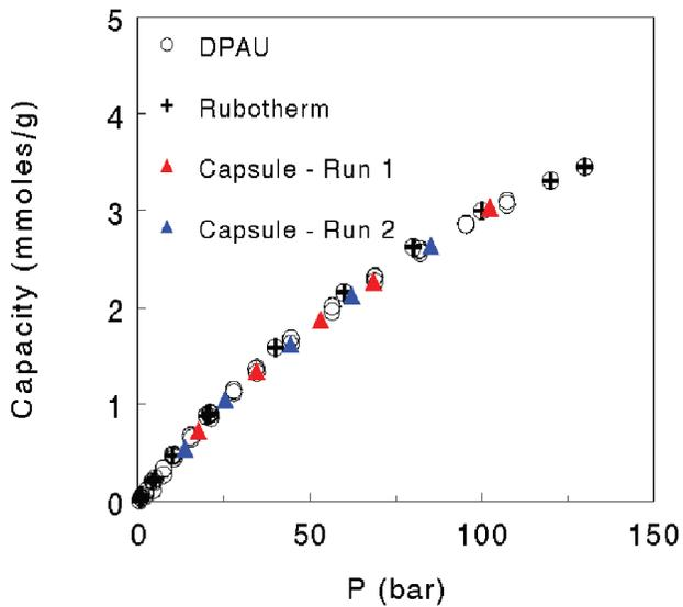
**FIGURE 2.** Overlay of hydrogen isotherms at 25°C for GX-31 activated carbon, comparing the results of the capsule method to our DPAU and a Rubotherm microbalance.
