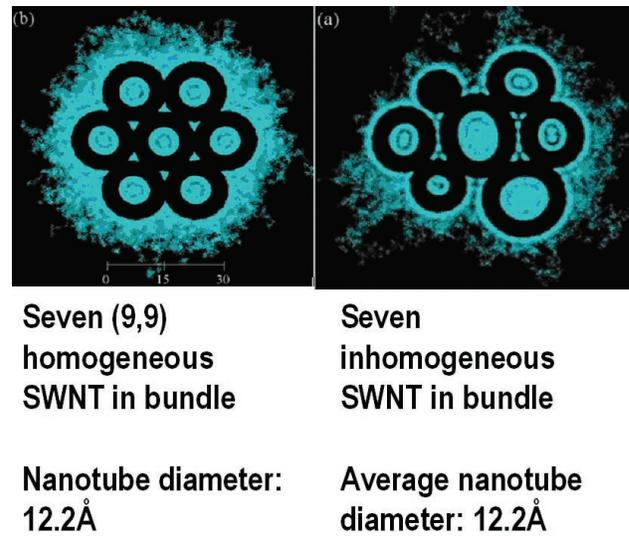
**FIGURE 3.** Plot of density of hydrogen in various regions in and around the homogeneous and inhomogeneous SWNT bundles during molecular dynamics simulations.
