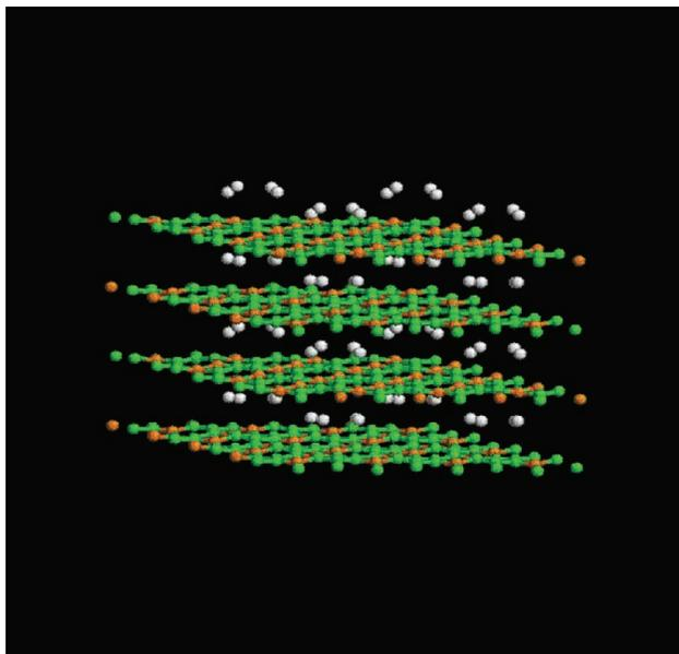
**FIGURE 4.** Snapshot of hydrogen adsorption on boron-doped graphite ( $C_{48}B_{16} \cdot 4 H_2$ ) during the molecular dynamics simulations (carbon-green, boron-orange, hydrogen-white).
