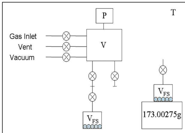
**FIGURE 1.** Illustration of Apparatus Used for Capsule Method Hydrogen Storage Measurements
