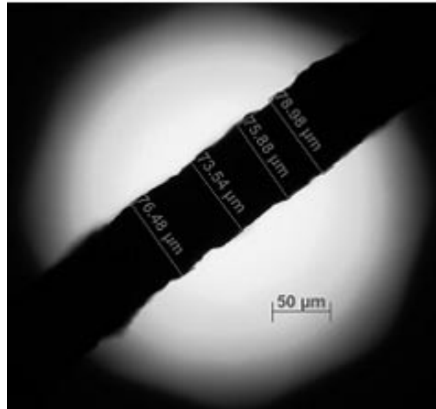
FIGURE 4. Fiber Before ( \sim 51 \mu\text{m} ) and After ( \sim 76 \mu\text{m} ) Swelling in Acid and Cross Linking With a Molecular Species, Showing the Fiber has Permanently Expanded by 50%.
